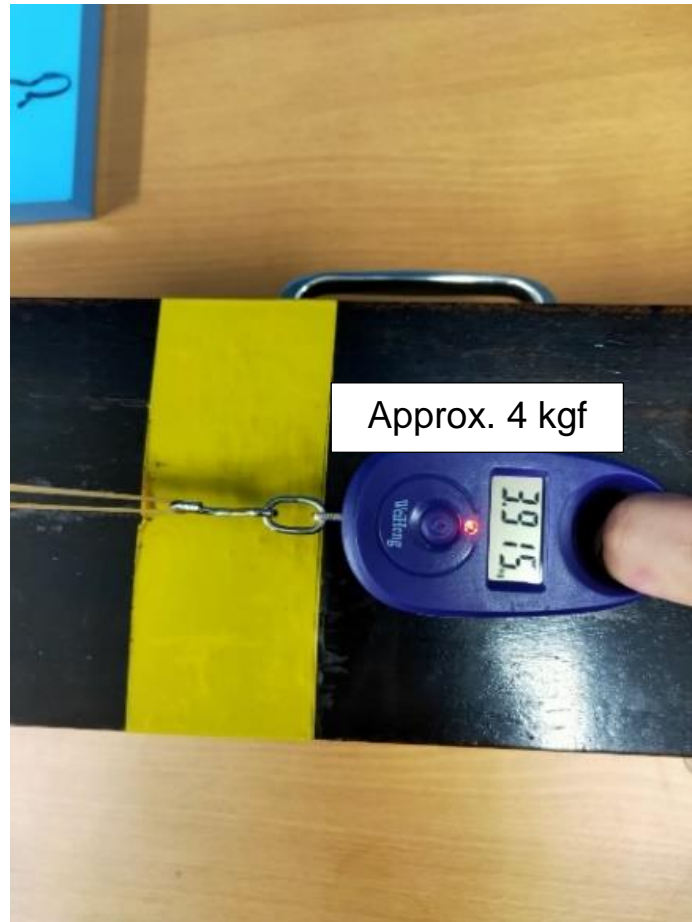
Figure 4: Unpowered Glider Launcher Launching Line
